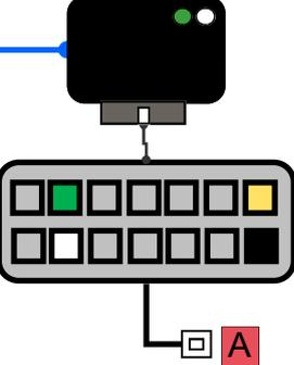
After making the connections, connect the Parking Sensor KIT BUZZER and the PARKVIEW wiring connector B and calibrate the Cobra system as usual.
