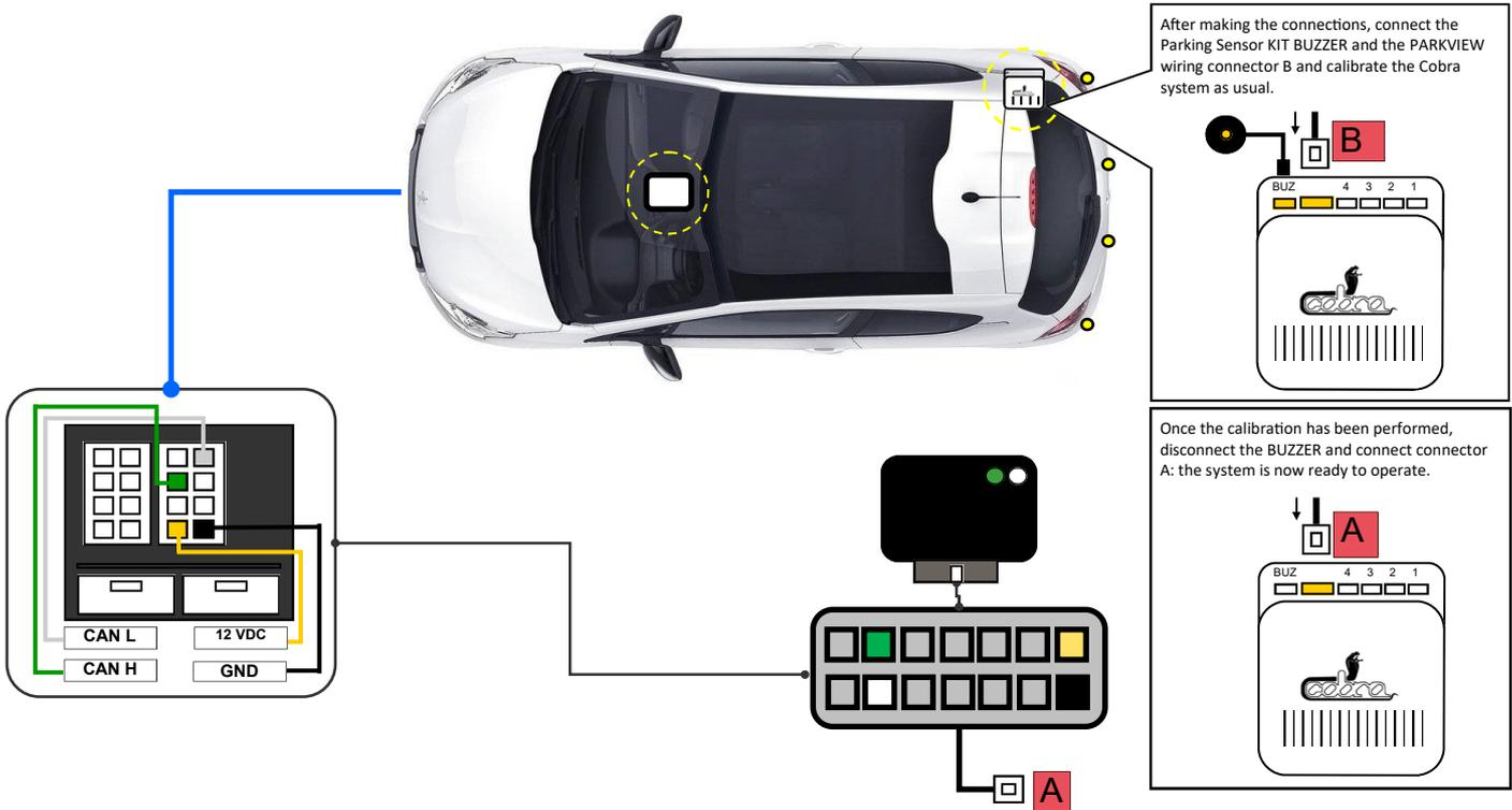
The harness supplied with PARKVIEW is split in 2 sections, the first is composed by 4 wires to connect on the radio compartment of the vehicle. Connect:
