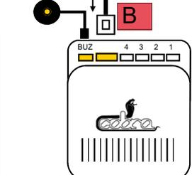
Once the calibration has been performed, disconnect the BUZZER and connect connector A: the system is now ready to operate.
