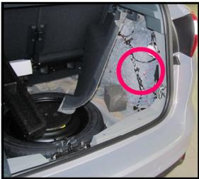
Remove the bulkhead in the trunk, behind it there are 3 connectors wrapped in a sponge
