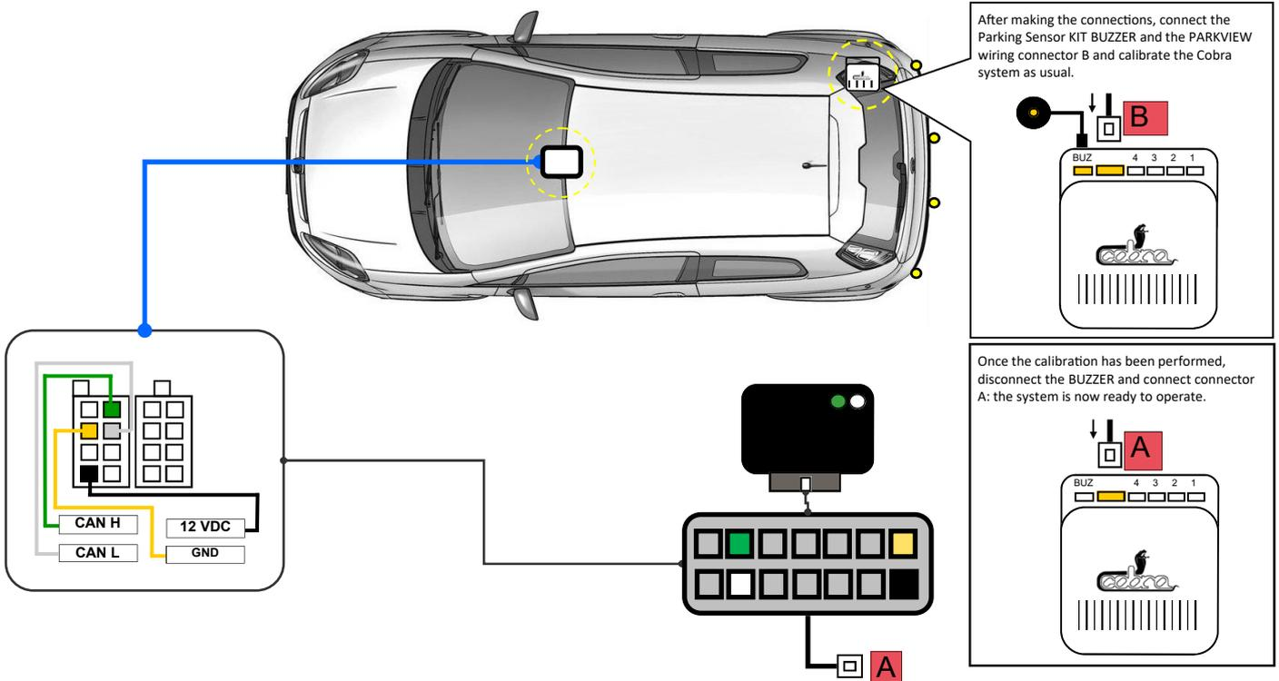
The harness supplied with PARKVIEW is split in 2 sections, the first is composed by 4 wires to connect on the radio compartment of the vehicle. Connect:
