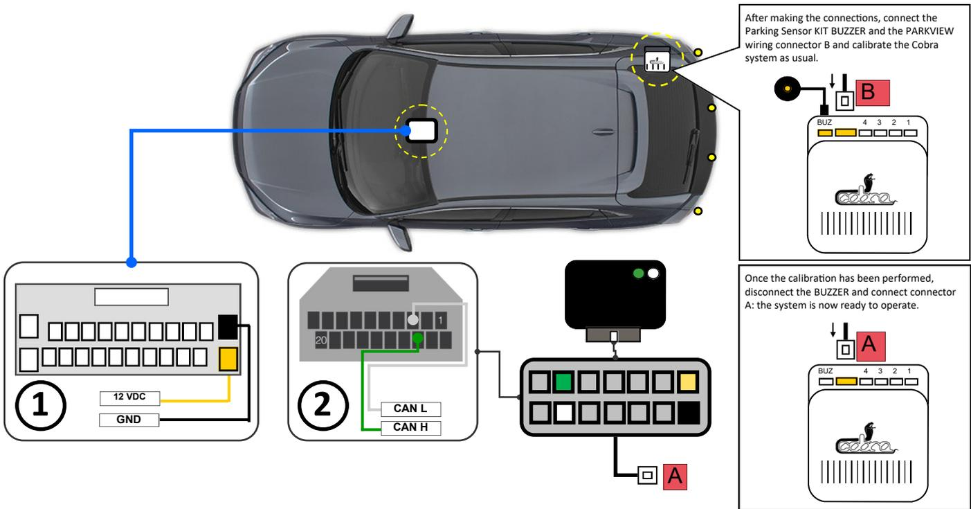
The harness supplied with PARKVIEW is split in 2 sections, the first is composed by 4 wires to connect to connectors 1 and 2 on the radio compartment of the vehicle. Connect:
