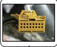
Once the calibration has been performed, disconnect the BUZZER and connect connector A: the system is now ready to operate.
