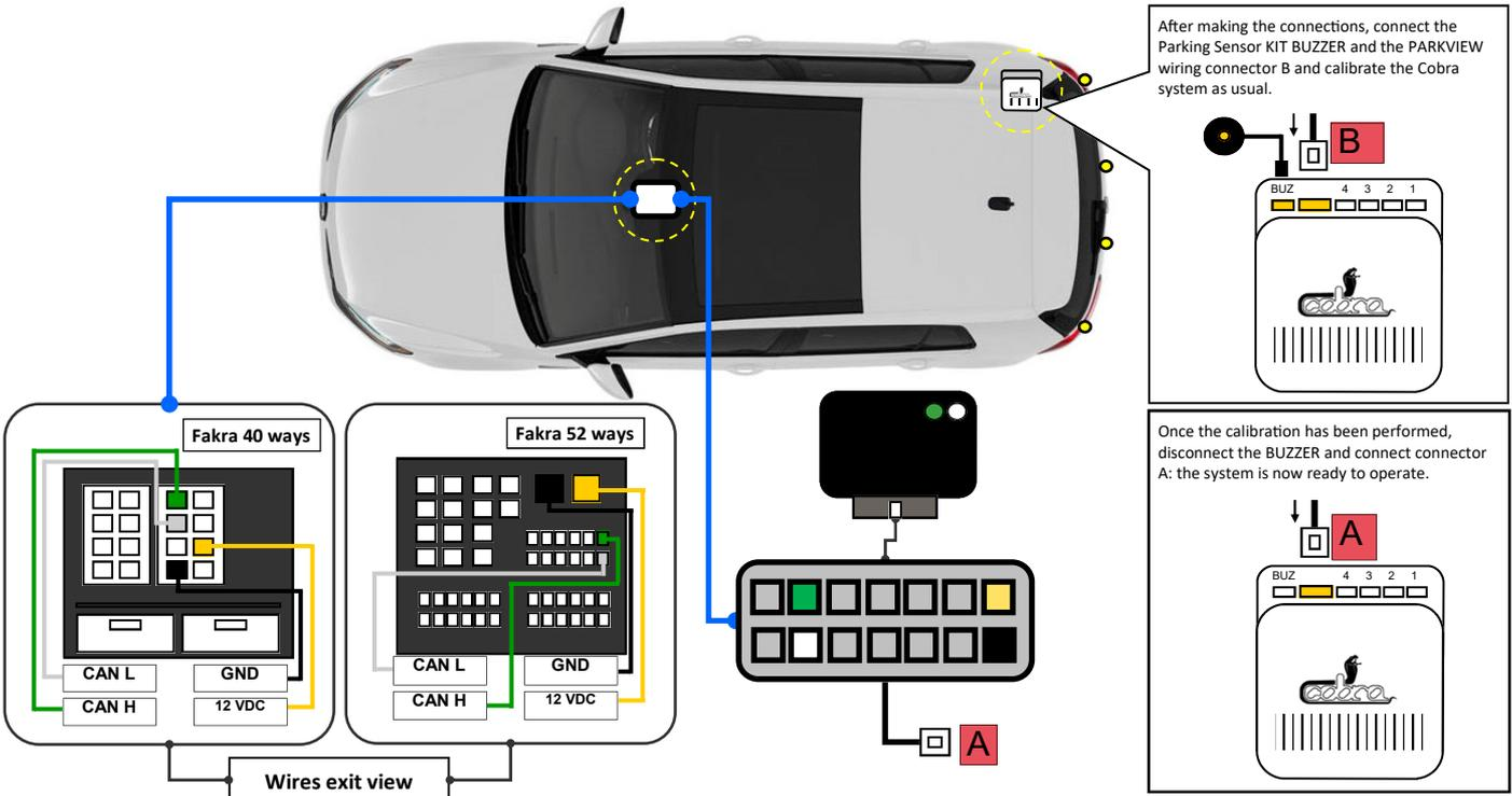
The harness supplied with PARKVIEW is split in 2 sections, the first is composed by 4 wires to connect back the OEM radio of the vehicle. In the FAKRA plug it must to connect:
