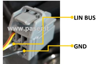
**POSIZIONE CONNETTORE: VANO RADIO - CONNECTOR LOCATION: RADIO SLOT**
