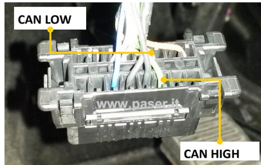
**POSIZIONE CONNETTORE ALTERNATIVA: VANO RADIO - ALTERNATIVE CONNECTOR LOCATION: RADIO SLOT**
