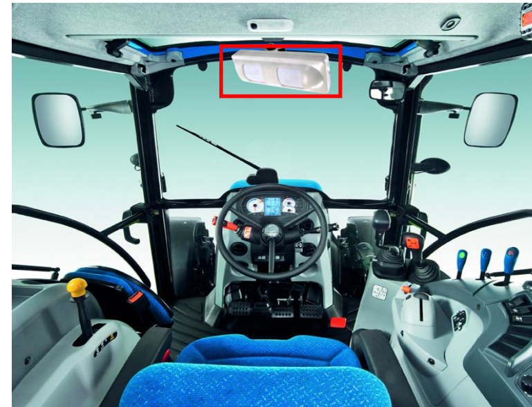
Mounting bracket for the sensor: if case of installation on the upper panel of the vehicle
