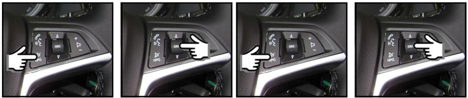
Entering the MENU is confirmed by a series of BEEPS from the buzzer. Now the buzzer will emit a BEEP followed by another BEEP. This means that we can set the first available function, i.e. AUTOMATIC FAN SPEED. Use the **SEEK** buttons to navigate the FUNCTIONS (use the WHEEL). Use the **VOLUME** buttons to navigate the SETTINGS. To confirm a setting, press **SOURCE**. Confirmation of the setting will be highlighted by a series of BEEPS from the buzzer.
