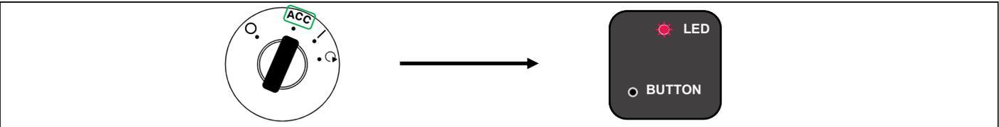
Now you must assign to each functions of your the aftermarket radio an available button/lever on your car steering wheel command. Functions assignment follows the sequential logic described in the TABLE below . The first function available is **VOLUME -** . Each time you press a button on your steering wheel, the UNICOM EVO JVC LED will briefly blink to indicate that the function has been correctly memorized
