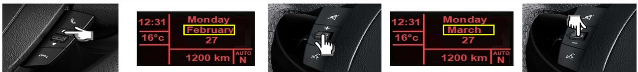
To turn to the DATE setting, press SEEK +. Volume buttons allow DATE adjustment. In this example the DATE is 27. To increase the day you need to press the button V+, to decrease it you need to press V-.
