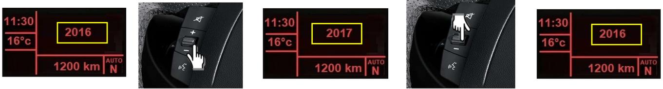
To turn to the HOURS setting, press SEEK +. Volume buttons allow HOURS adjustment. In this example is 11:30. To increase hours you need to press the button V+, to decrease them you need to press V-.
