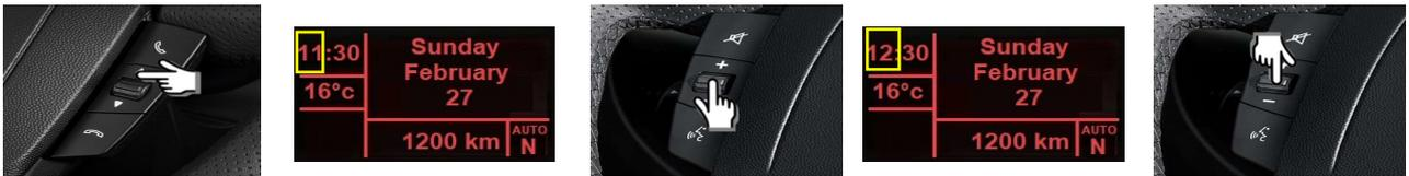
To turn to the MINUTES setting, press SEEK +. Volume buttons allow MINUTES adjustment. In this example is 11:30. To increase minutes you need to press the button V+, to decrease them you need to press V-.
