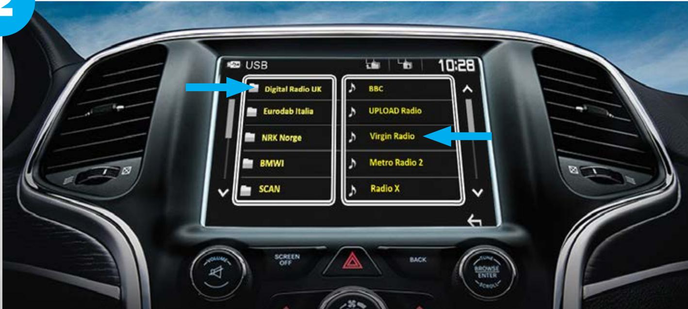
Selected USB function, the radio will display the folders that will be named according to the MUXs in the coverage area. By selecting the various MUXs will have the list of available stations. By selecting a station of interest, it will proceed with listening.
