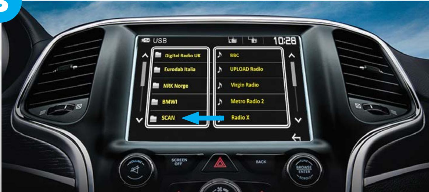
**It is recommended to run a SCAN for the correct reception of the MUXs and stations present in the signal coverage area. This operation is very simple: you only have to select SCAN by radio commands or press and keep pressed the SERVICES BUTTON till the scanning starts; Signal scan will start immediately signalled by an acoustic ring. This takes about 2 minutes.**
