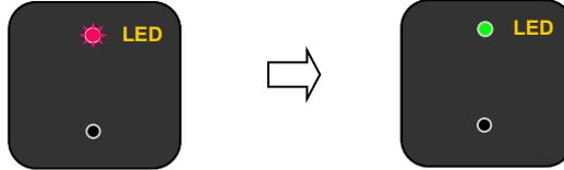
Plug the REMOTE adapter back the radio. The unit is ready to work.
