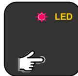
To exit the procedure, you must press and keep pressed one of the memorized buttons till the LED light YELLOW. As soon as you release the button, LED will light GREEN. Plug the REMOTE adapter back the radio, unit is ready to work.
