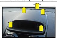
Now rotate the display so to have the acces to the connector of the display.
