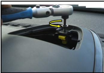
Once the torques is removed, detach the display with its plastic .
