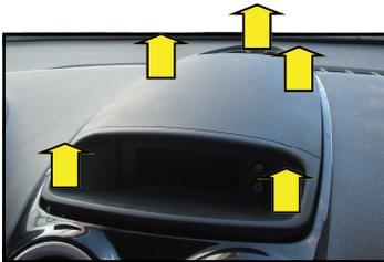
Now rotate the display so to have the acces to the connector of the display.
