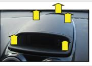
Now rotate the display so to have the acces to the connector of the display.
