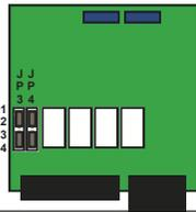
If the vehicle is equipped with an OEM amplifier (booster) please set the jumpers as described in the picture beside. We suggest that if it's possible to connect the unit to an external speaker. Also with the external speaker follow the jumper setting of the picture.
