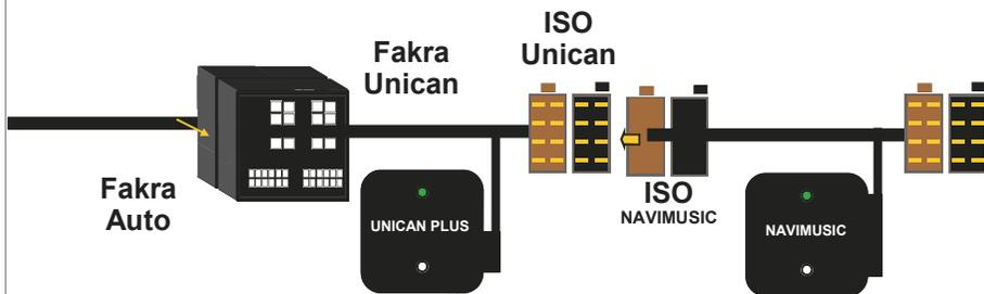
Connect the Navimusic ISO connector to the aftermarket radio ISO connector. Connect the UNICAN PLUS plug adapter (for the radio functions control) to the dedicate input located back the aftermarket radio. Connect the YELLOW WHITE wire as below described.
