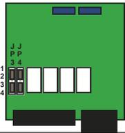
If the vehicle is equipped with an OEM amplifier (booster) please set the jumpers as described in the picture beside. We suggest that if it's possible to connect the unit to an external speaker. Also with the external speaker follow the jumper setting of the picture.
