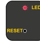
Done the synchronization, it is selected the car protocol; this operation is confirmed by the Turning on **GREEN** of the module led, that will start to light. The unit is ready to SELECT THE AUTORADIO.
