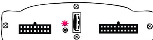
Making the sincronization the car protocol is selected, this operation is confirmed when the **FIXED GREEN** on the module LED switch on.
