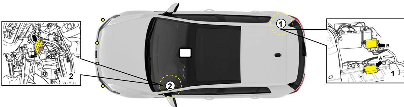
Once the location of the original parking sensor control unit has been identified, it is necessary to disconnect the brown connector A, then connect the kit wiring in series between the OEM connector and the original parking sensor control unit B.
