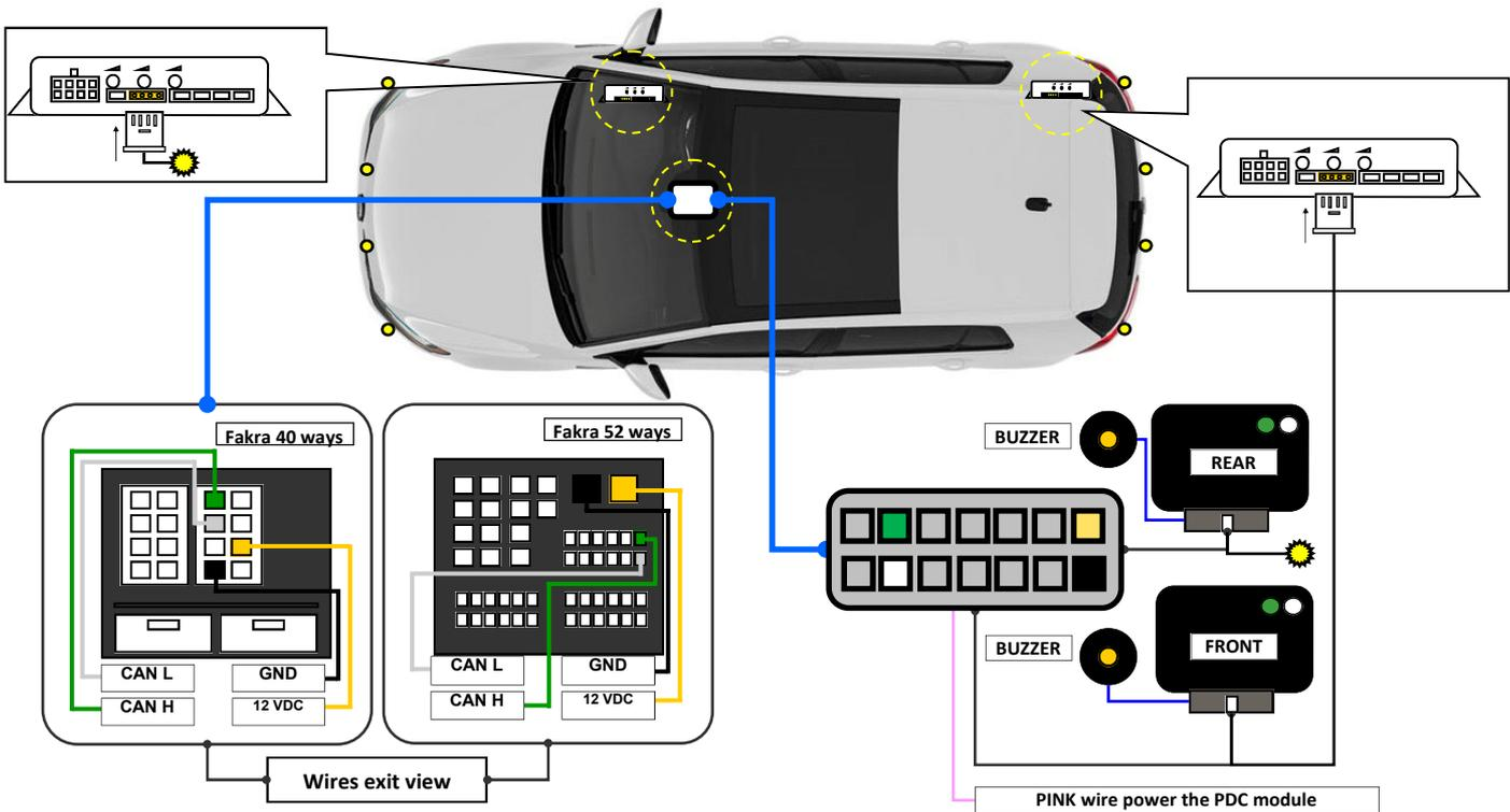
The harness supplied with PARKVIEW is split in 2 sections: the first is composed by 4 wires to connect back the OEM radio of the vehicle. In the QUADLOCK plug it must to connect:
