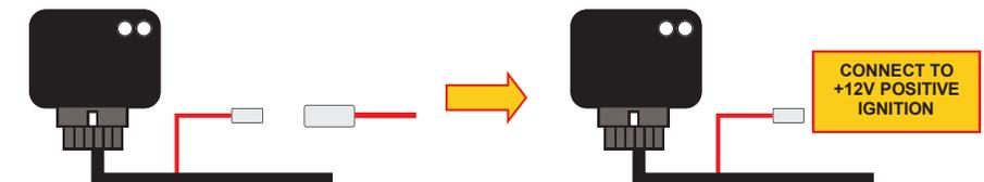
Break red wire connection between interface and OBD port.
