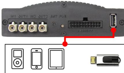
Reproduction will start automatically after the device connection, anyway it will be always possible to change the active source by the interface menu.
