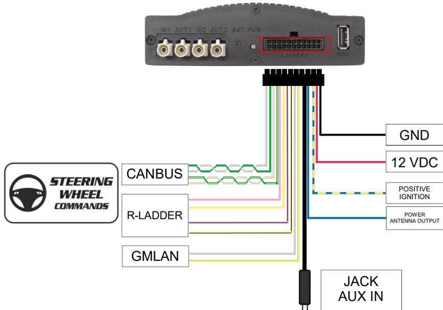
**Connect steering wheel interface wires in series to the car that uses CANBUS protocol is necessary to cut the GREEN wire to the car side and GREEN/YELLOW to the radio side, the same must be done with CAN L and WHITE and WHITE/YELLOW wires.**
